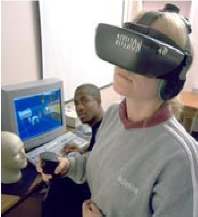
**Sistema VR: Display HMD (Head Mounted Display)
